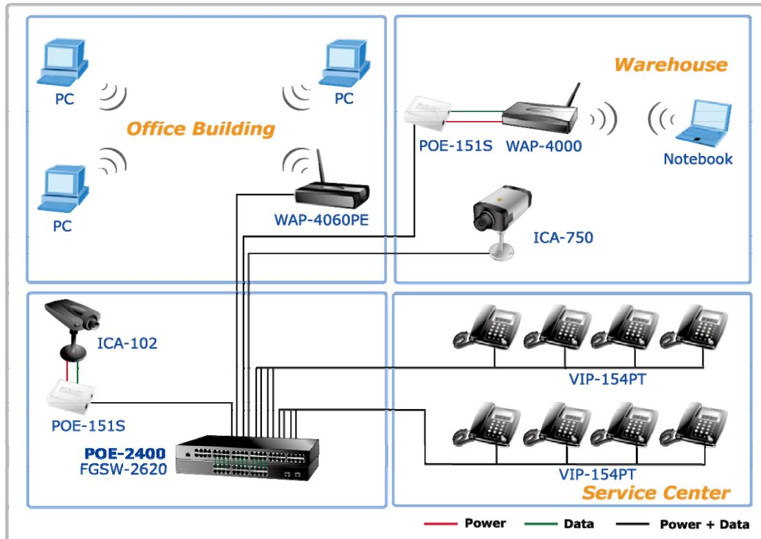
Figure 1-1 Power over Ethernet Application
