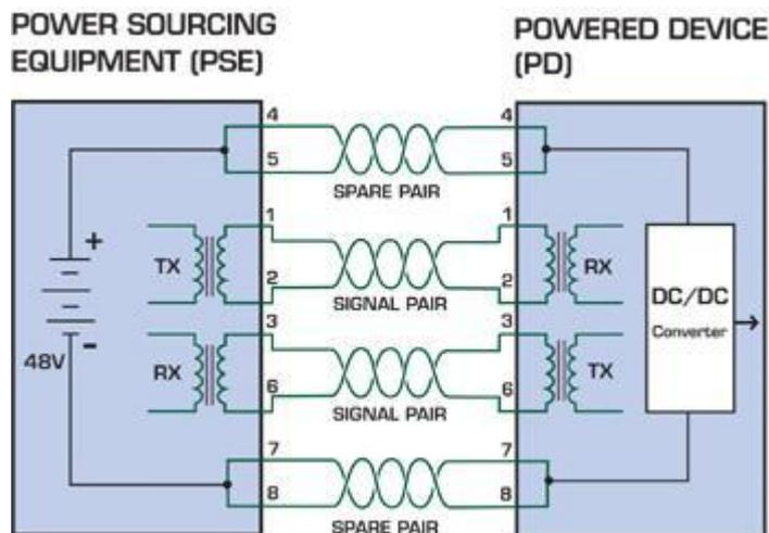
Figure 2 - Power Supplied over the Spare Pins
