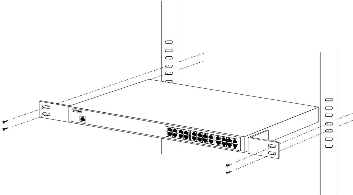
**Figure 2-6** Mounting the PoE Injector Hub in a Rack
