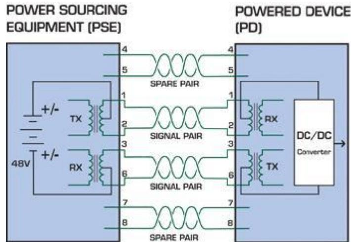
Figure 3 - Power Supplied over the Data Pins
