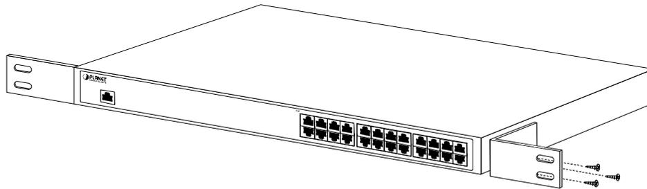
**Figure 2-5** Attaching the brackets to the PoE Injector Hub
