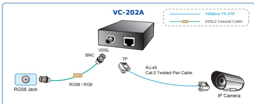
**Figure 3-6:** Connecting Standalone IP Device
