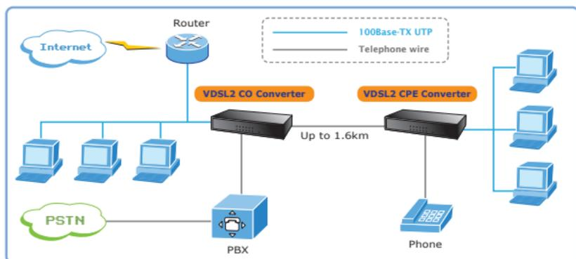
**Figure 3-2:** VC-204 LAN to LAN Connection
