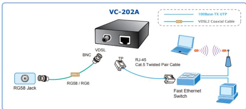
**Figure 3-7:** Connecting Multiple PCs to an Ethernet LAN
