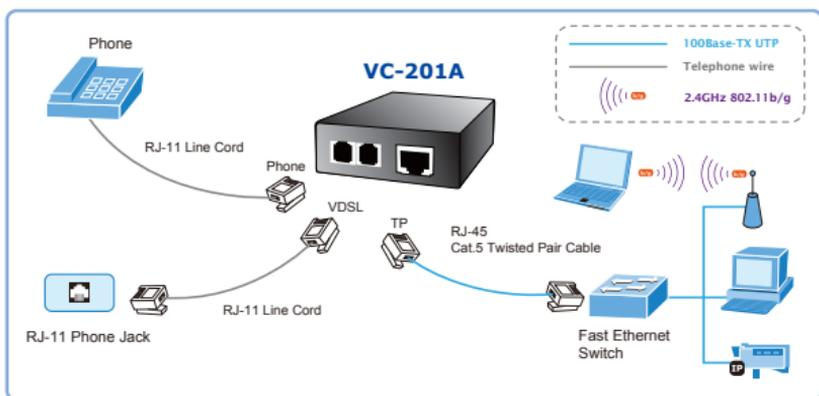
**Figure 3-5:** Connecting Multiple PCs to an Ethernet LAN
