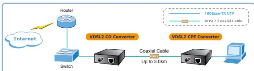
**Figure 3-3:** VC-202A LAN to LAN Connection
