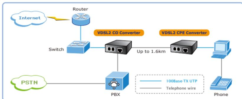
**Figure 3-1:** VC-201A LAN to LAN Connection
