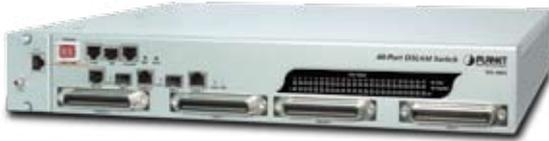
The PLANET IDL-4802 is a 48-Port ADSL/ADSL2/ADSL2+ mini IP DSLAM which equips with combo electrical (RJ-45) and fiber optical (SFP) uplink interfaces offering scalable and easy deployment for the network with small ADSL environment. With the built-in POTS splitter subscriber ports, the IDL-4802 performs a cost-effective solution for network service providers to offer multiple subscribers excellent services.
