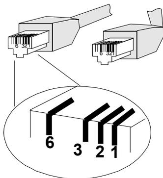
There are 8 wires on a standard UTP/STP cable and each wire is color-coded. The following shows the pin allocation and color of straight cable and crossover cable connection:
