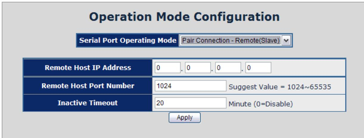
Figure 4-49 Pair Connection – Remote (Slave) Configuration screen
