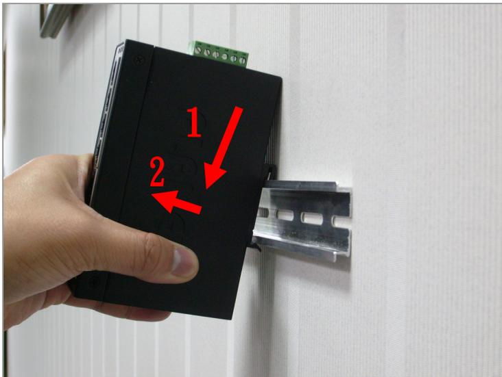
**Figure 2-10** Remove Industrial Equipment in DIN-Rail mount.
