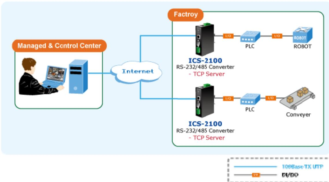
**Figure 1-2** Industrial Serial Converter for Factory PLC Application
