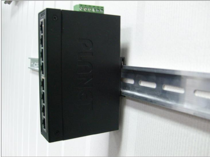
**Figure 2-9** Industrial Equipment installed in DIN-Rail mount.
