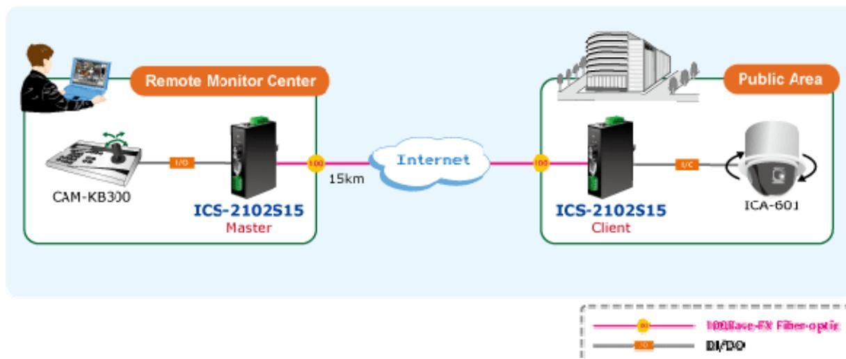
Figure 1-4 Industrial Serial Converter for Distance Extend Application
