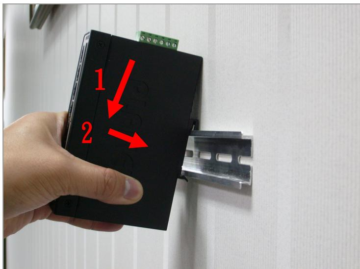
Figure 2-8 Install Industrial Equipment in DIN-Rail mount.
