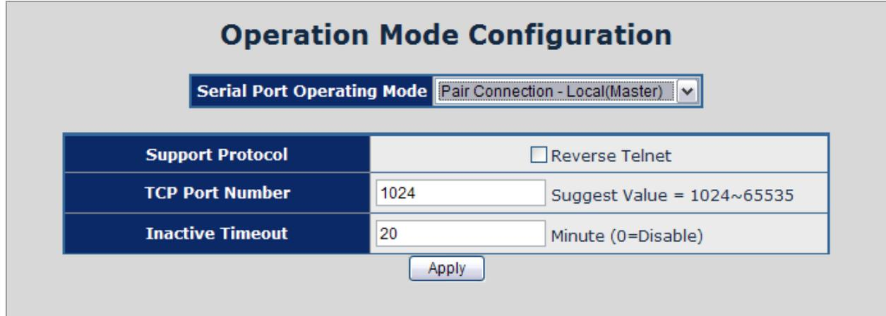
Figure 4-48 Pair Connection – Local (Master) Configuration screen
