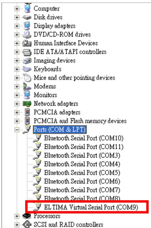
Figure 5-11 Windows Device Server - Virtual COM Port
