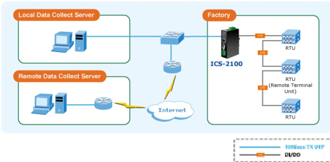
**Figure 1-3** Industrial Serial Converter for Factory RTU Application
