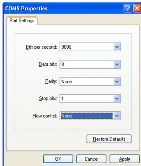
Figure 4-35 Example: HyperTerminal COM port properties screen
