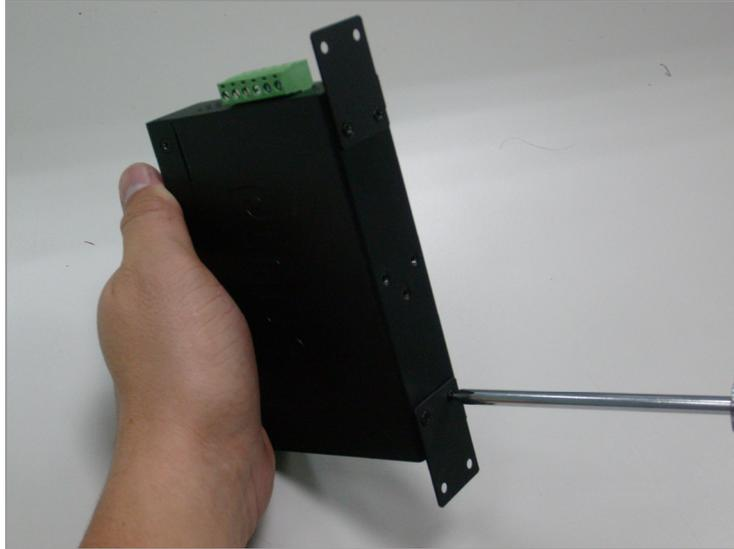
**Figure 2-11** Attach brackets to the Industrial Equipment.
