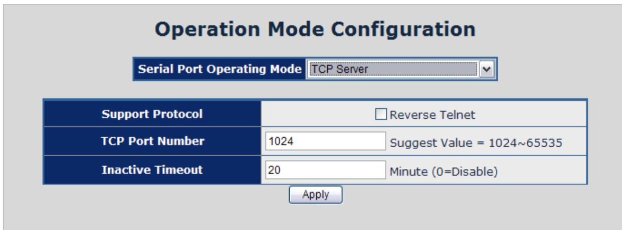
Figure 4-15 Example: TCP Server Configuration screen
