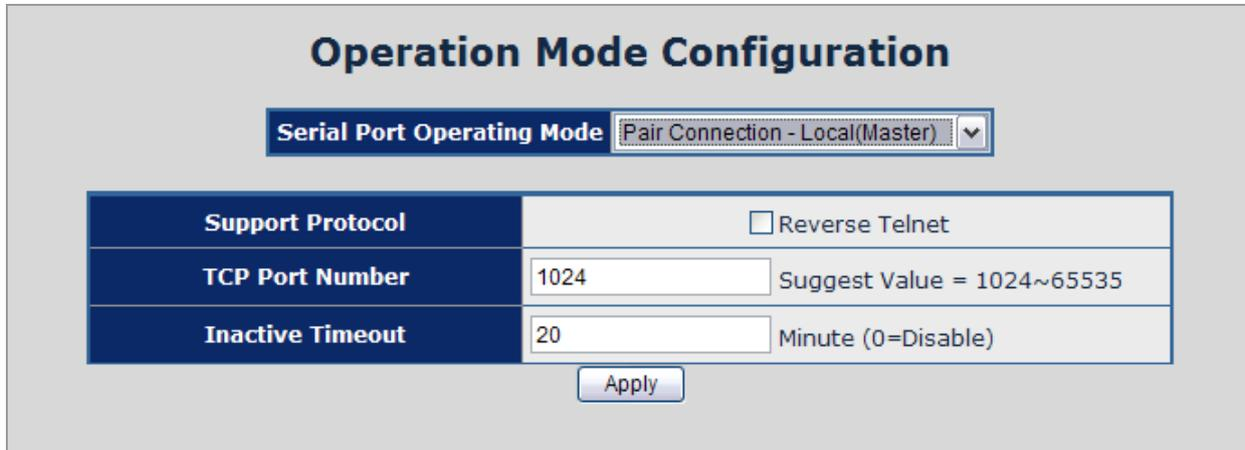
Figure 4-51 Pair Connection – Local, operation mode configuration
