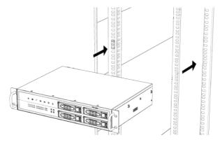
• Lock the server to the rack by mounting the ear brackets to the rack.
