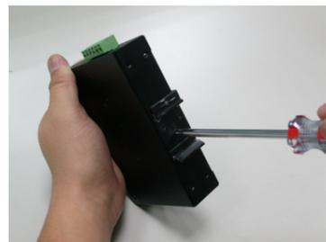
**Step 1:** screw the DIN-Rail on the Industrial Fast Ethernet Switch.
