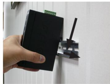
**Step 2:** Lightly press the button of DIN-Rail into the track.
