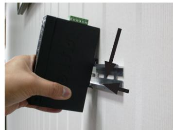
**Step 5:** Lightly press the button of DIN-Rail for remove it from the track.
