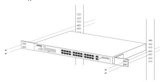
Figure 4: Mounting the Fast Ethernet Switch in a Rack
