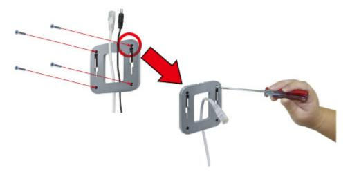
Figure 3-1 WNAP-C3220 Installation Diagram 1
