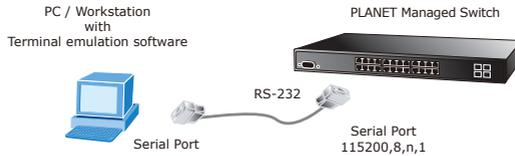
A terminal program is required to make the software connection to the Managed Switch. Windows' **Hyper Terminal** program may be a good choice. The Hyper Terminal can be accessed from the **Start** menu.
