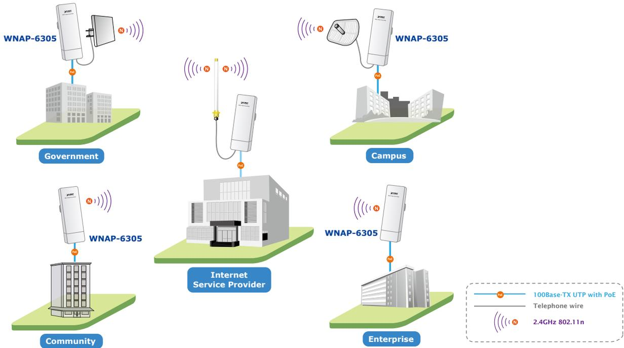
With built-in RP-SMA type Antenna connector and high output power with multiple adjust Tx controller, the WNAP-6305 provides higher coverage and longer distance wireless connection, and also allows CPE users to easily install and adjust the suitable value in appropriate locations. The WISP mode supported enables CPE users to connect to Internet via local WISP provider.
