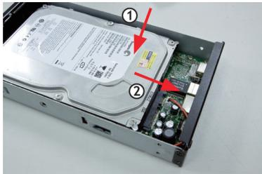
1-3. Secure the HDD with the HDD screws at both ends.
