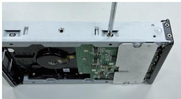
1-4. Push the tray back into the case and tighten the bottom screws.
