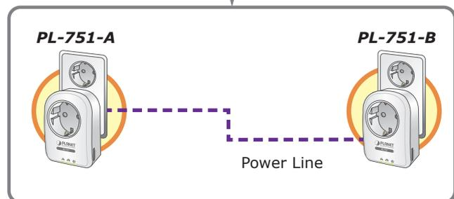
**Step. 3** Connect the PC via the network cable to the Powerline Ethernet bridge.
