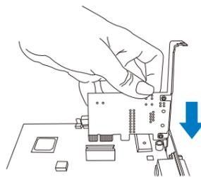
**Step 6:** Secure the Gigabit Ethernet Adapter with the screw you saved in step 4.
