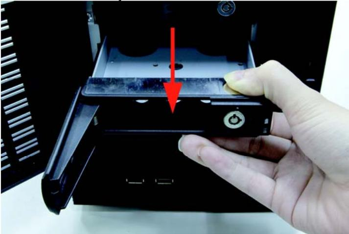
3. Place the HDD in the tray by unscrewing and screwing it.
