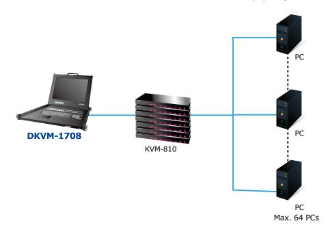
The Combo-Free KVM can be connected to any PC or server directly without concern of keyboard / mouse interface compatibility.
