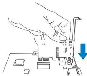
**Step 6:** Secure the 10 Gigabit Ethernet Adapter with the screw you saved in Step 4.
