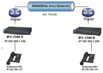
Step1: Configure the mapping rule of IPX-2500-A on the router.
