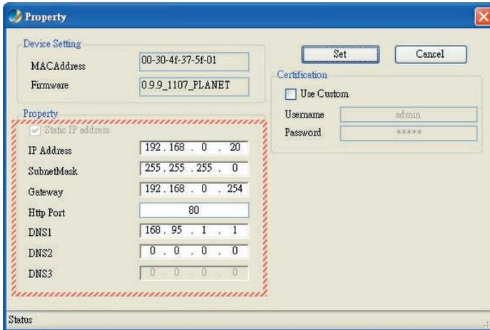
4. After filling the desired settings in the properties, click on “Set” button to complete the configuration settings.
