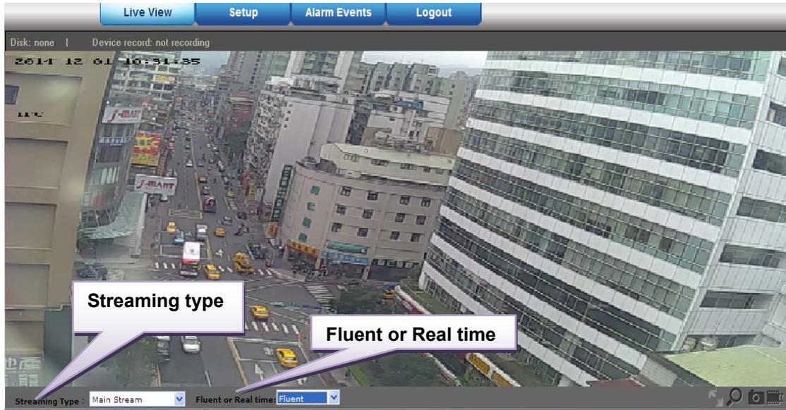
**Streaming type** Set up the real time view stream type (Main stream/Sub stream).
